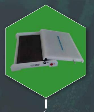
For the first time in 1984, Andersen introduced the Semi-Dry Blotting technique. Initially, the blotting technique was performed horizontally, using plate electrodes. The gel and nitrocellulose membrane were sandwiched between layers of wetted filter paper.
