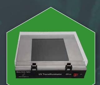
The UV transilluminator **is** the simplest method for high-quality visualization of DNA bands. After completing the electrophoresis process, it is necessary to examine the results related to the DNA bands.
